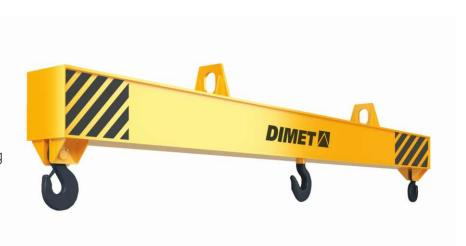
**DIMET hook linear beams** are used for handling various long loads when the lifting height is restricted. The beam design may include reversible cages or extendable cantilevers used to adjust the distance between cargo attachment points. This design is used when it is required to handle cargoes of various length. Depending on the type, we equip beams with various grips:
